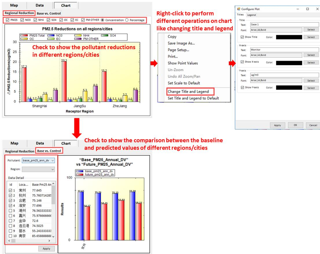
Fig. 24 Chart results and configuration options of SMAT-CE
