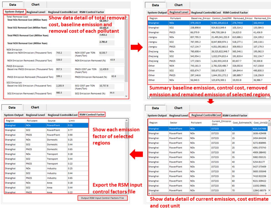
Fig. 17 Data detail results and configuration of ICET
