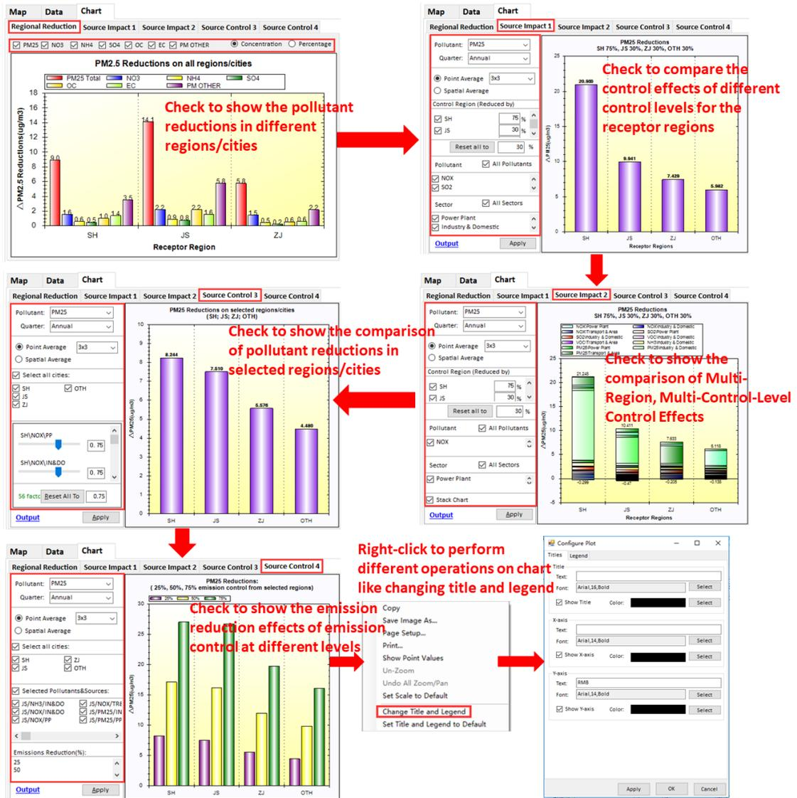
Fig. 21 Chart results and configuration options of RSM-VAT
